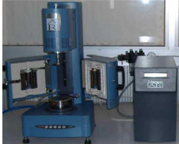
Fig.2 Rheometer AR 2000
