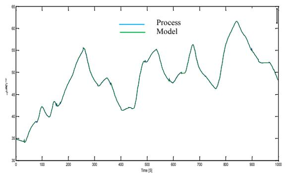
Fig. 5. Process and fuzzy model outputs on  $T_{34}$  testing data
