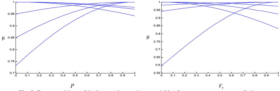
Fig. 2. Fuzzy partitions of the heat exchanger input variables for water temperature prediction.
