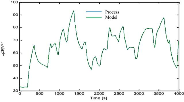
Fig. 3. Process and fuzzy model outputs on  $T_{34}$  training data
