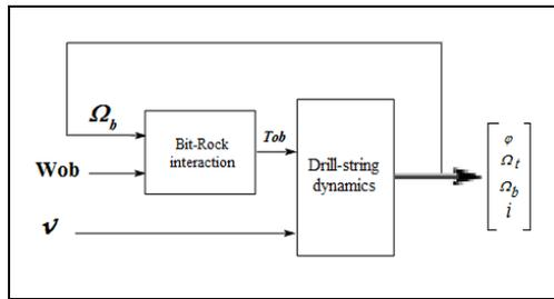
Figure 3. Block diagram of a torsional model of the drill-string
