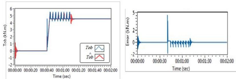
Figure 10. Torque-on-bit and Torque-on-bit estimation (on the left). estimation error of Tob (on the right)
