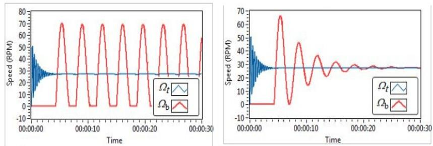
Figure 7. Angular velocity of the BHA ( $\Omega_b$ ) and the speed at the surface ( $\Omega_t$ ) under ( $\omega_{ob}=15T$ ) and ( $v=125V$ ). Top : with ( $C_t=51.38 Nms/rad$  ,  $C_b=39.79 Nms/rad$ ), Bottom: with ( $C_t=63,54 Nms/rad$  ,  $C_b= 56,85 Nms/rad$ )
