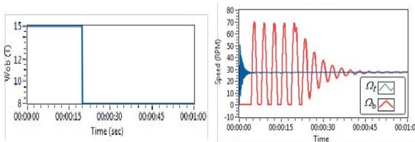
Figure 6. Angular velocity of the BHA ( $\Omega_b$ ) and the speed at the surface ( $\Omega_t$ ) under a constant DC motor voltage ( $v=125V$ ) and decreasing weight-on-bit from ( $Wob=15T$ ) to ( $Wob=8T$ ) at ( $t=20s$ )
