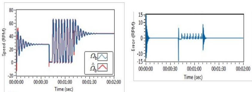
Figure 9. BHA speed and BHA speed estimation (on the left). estimation error of the speed at the surface (on the right)
