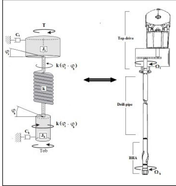
Figure 1. Mechanical model describing the torsional behavior of a generic drill-string.
