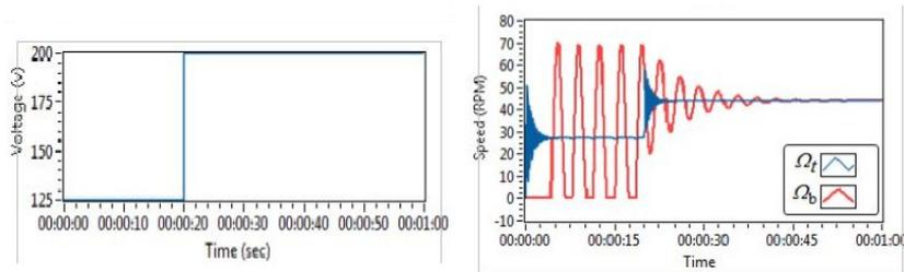
Figure 5. Angular velocity of the BHA ( $\Omega_b$ ) and the speed at the surface ( $\Omega_t$ ) under a constant weight-on-bit ( $Wob=15T$ ) and augmentation of DC motor voltage from ( $v=125V$ ) to ( $v=200V$ ) at ( $t=20s$ )
