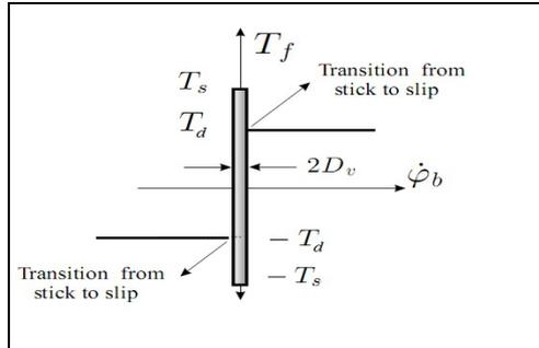
Figure 2. Models for the friction between the bit and the rock given by expression (9)
