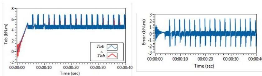
Figure 13. Torque-on-bit and Torque-on-bit estimation (on the left). Estimation error of Tob (on the right)
