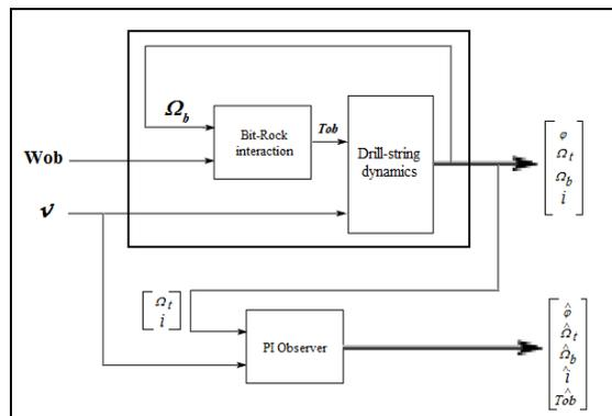
Figure 4. Block diagram of a PI Observer for unknown input.
