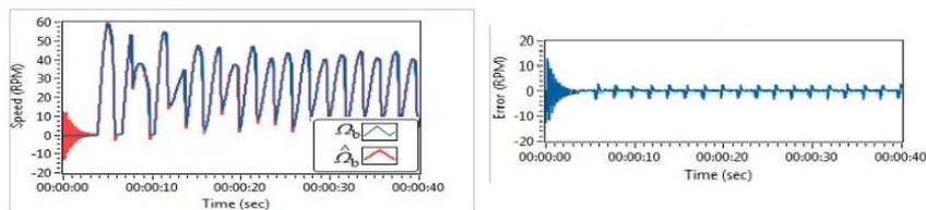
Figure 12. BHA speed and BHA speed estimation (on the left). Estimation error of the speed at the surface, under Wob shown in figure 12 and motor voltage =125V (on the right)
