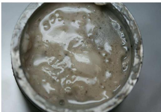
Figure 6. Filter cake on front of sample rock.
