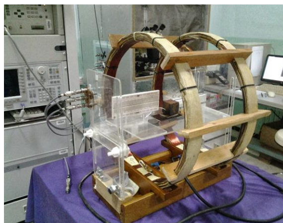
Fig. 1. Photo of a Helmholtz coil used to generate uniform magnetic field
