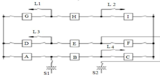
**Figure 7:** a breaker and a half substation configuration with labeled components
