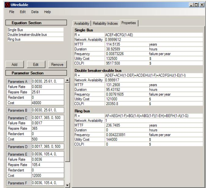
Figure 6: Reliability assessment results for single bus, double breaker-double bus and ring bus
