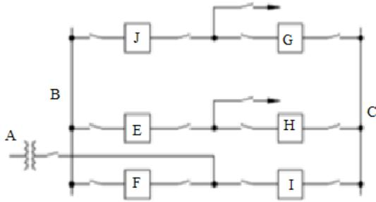
Figure 4: Double breaker-double bus labeled components
