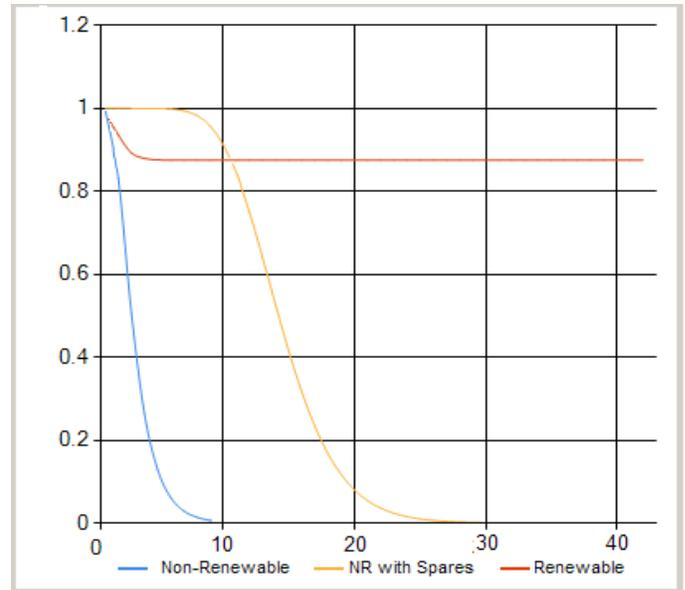
**Figure 9:** plot of a non-renewable (with and without spares) and a renewable behavior of breaker and a half substation
