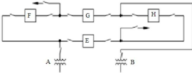
Figure 5: Ring bus labeled components.
