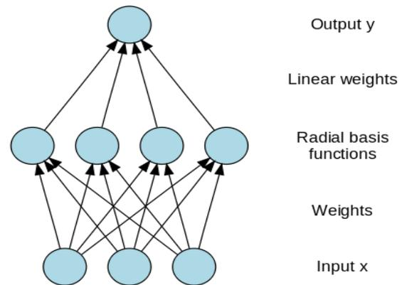
Figure 01 An example of a RBF neural network with three inputs and one output
