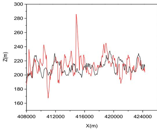
Figure 10 Denoised GPR profile (red color) compared with the same profile free of noise (black color)
