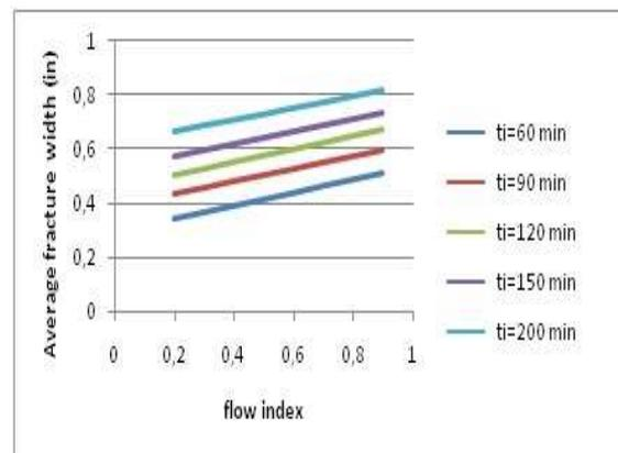
Fig. 2: Average fracture width versus power law exponent for different ti
