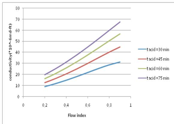
Fig.8 Conductivity as a function of flow index
