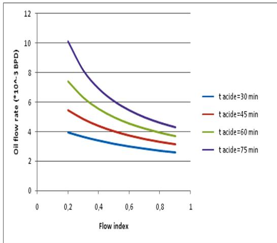
Fig.5 Oil flow rate as a function of flow index
