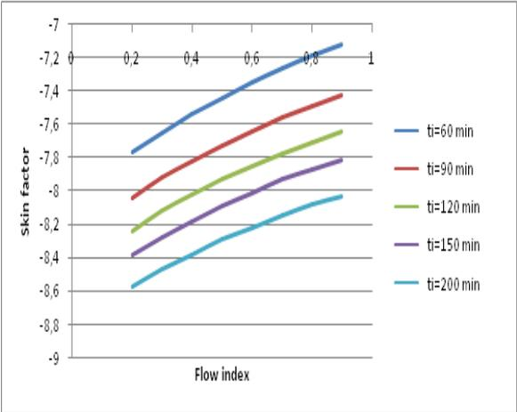
Fig.3 Variation of the pseudo-skin of the fracture as a function of the flow
