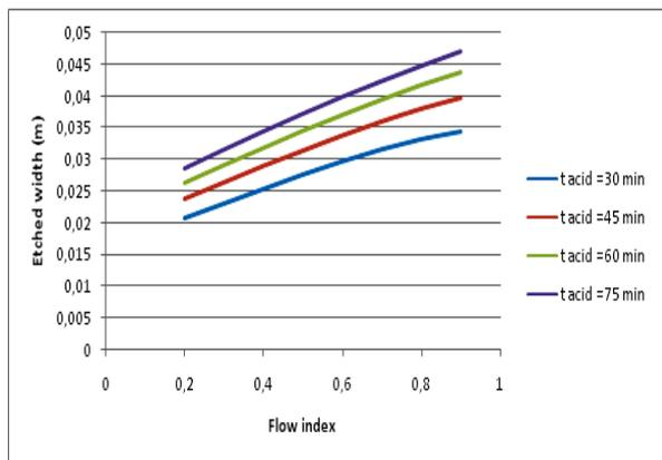
Fig.7 Etched width as a function of flow index
