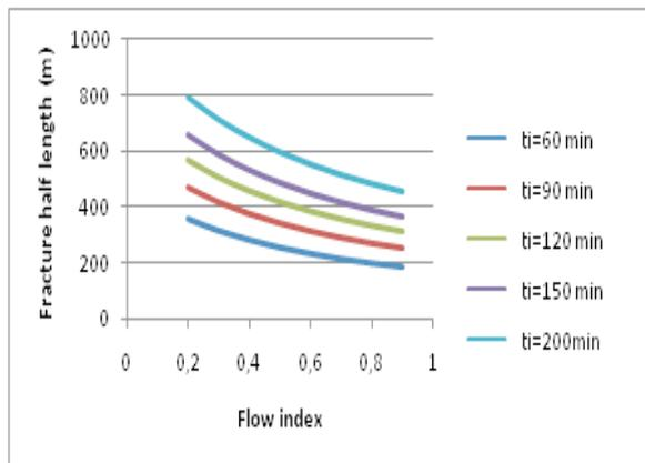
Fig.1 Fracture half length as a function of flow index for different ti
