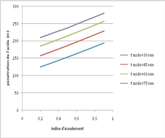
Fig.4 Acid penetration as a function of flow index
